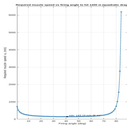
**Figure 5.** Required muzzle speed vs firing angle (Quadratic drag) to hit 1200 m
