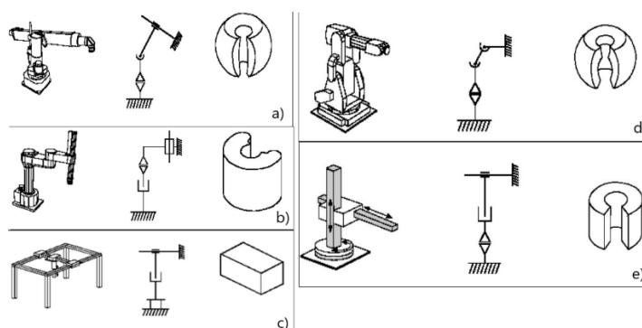
**Figure 1.** Types of kinematic structures and shapes of their workspaces; a) spherical robot, b) SCARA robot, c) cartesian robot, d) cylindrical robot, and e) angular robot.
