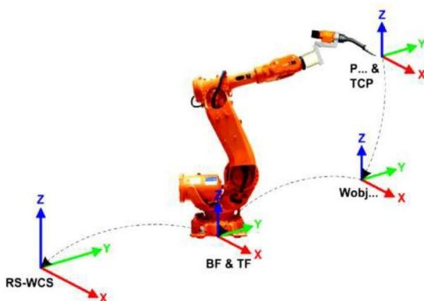
**Figure 5.** Coordinate systems of industrial robots (ABB Robotics, 2010).
