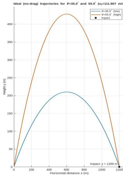
**Figure 2.** Ideal trajectories for  $\theta = 35.0^\circ$  and  $55.0^\circ$  ( $V_0 = 111.907$  m/s)
