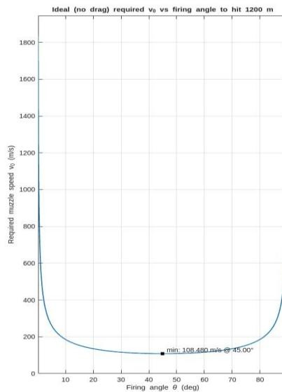
**Figure 1.** Ideal required  $V_0$  vs Firing angle to hit 1200 m
