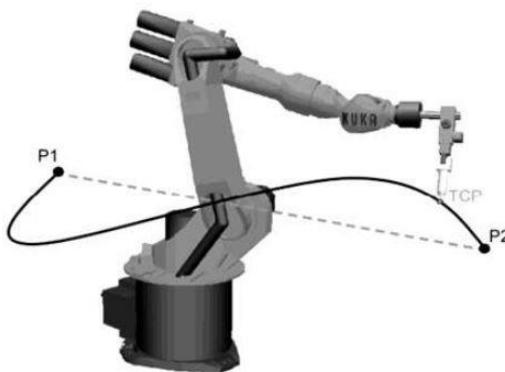
**Figure 2.** General movement of an industrial robot (Pochylý, 2012).
