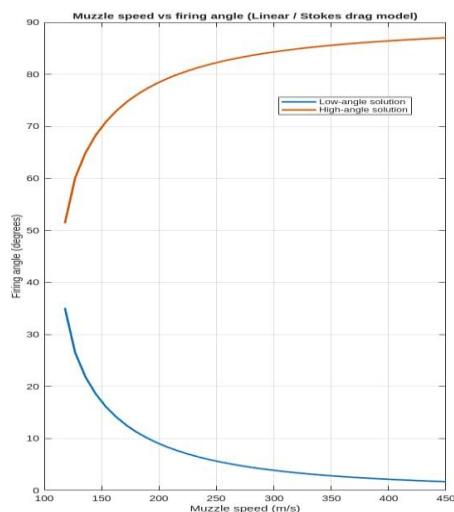
**Figure 3.** Muzzle speed vs firing angles (linear drag model) to hit 1200 m
