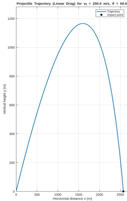
**Figure 4.** Projectile Trajectory (Linear drag model) for  $V_0 = 250.0$  m/s,  $\theta = 50.0^\circ$
