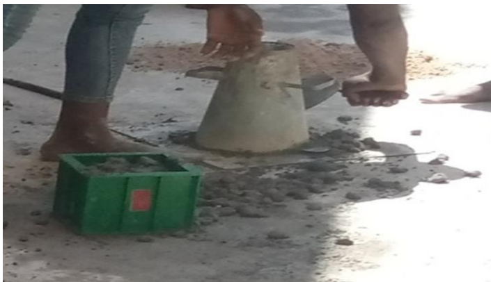
Figure 3. Photograph of Procedure of Slump Test and Casting of cubes
