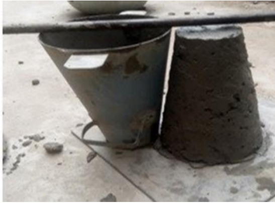
Figure 4. Photograph of Slump Test Specimen and Cone
